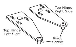
1. Remove pivot screw from hinge, flip hinge over, and install the pivot screw in the same hole from the opposite surface.
