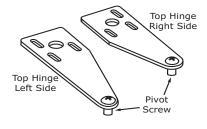
1. Remove pivot screw from hinge, flip hinge over, and
