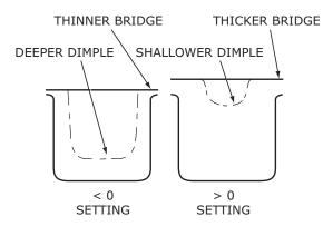
Ice thickness adjustments are made using the control panel as follows:
