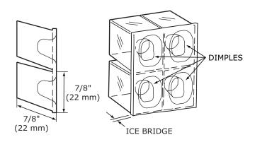
Your clear ice machine is preset to produce ice between the optimal dimensions illustrated below:
