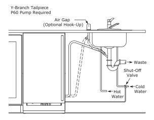
The maximum lift for the P60 drain pump is 10 feet. This must be done as close to the rear of the unit as possible.
