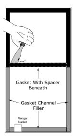
4. Take out 2 screws and remove plunger bracket from gasket channel.
